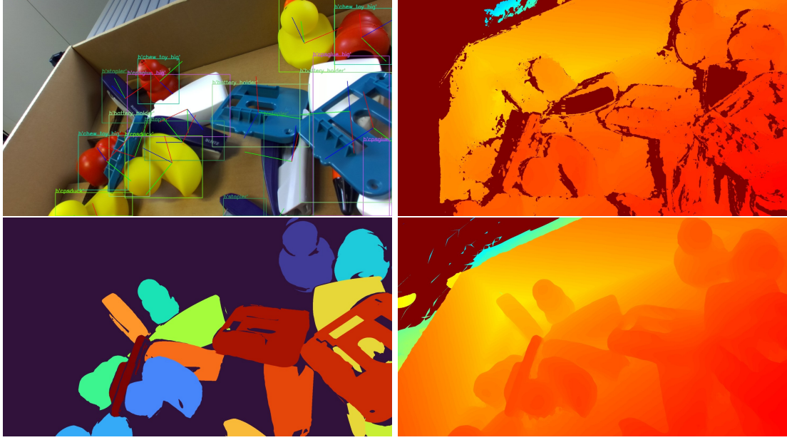
Figure 12: One sample from our real dataset. From left to right, the annotated RGB image, the depth images of the camera, the segmentation mask, and the high-quality restored depth image are shown for the left camera of the stereo camera.
