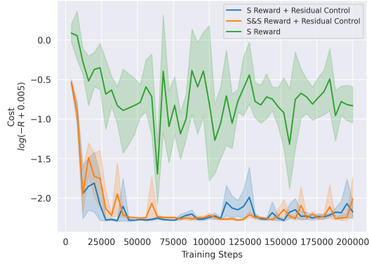
Figure 5: The plot illustrates the training progress with and without residual mechanisms. In the residual control diagram, the model-based control guides the exploration of the DRL, significantly improving the converging speed and leading to the enlarged reward (reduced cost).
