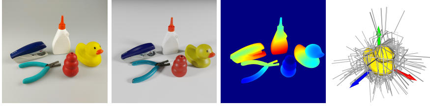
Figure 21: From left to right: the five selected objects photographed, photo-realistically rendered, depth rendered and automatically generated grasp poses for the duck.
